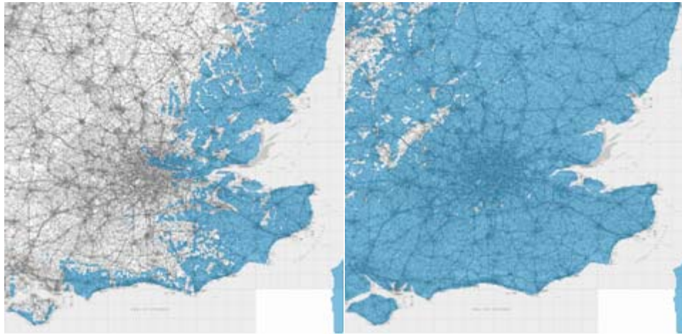
Exhibit 3.9: Illustration of interference contour from Continental DTT transmitters on Channel 65 for 50% of time (left) and 1% of time (right) [Source: Aegis]
