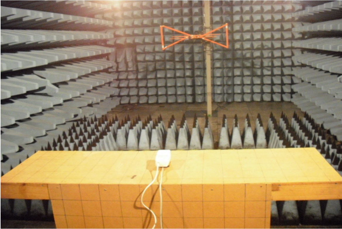
Photograph 2: Radiated Emissions pre-scan
