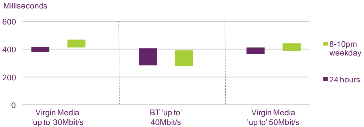
Figure 34 Average and peak time loading of web pages for above ‘up to’ 24Mbit/s packages, November 2011
