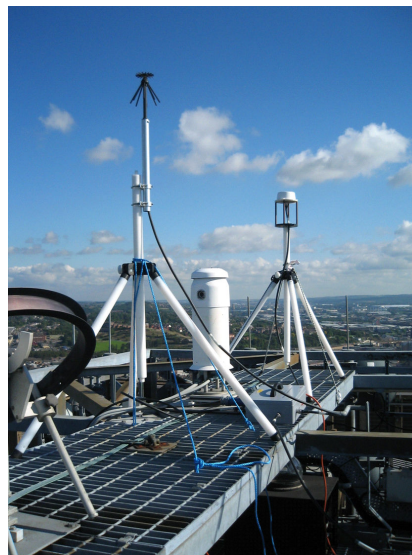
Figure 9 AIMS monitoring LE bands at Sheffield University
